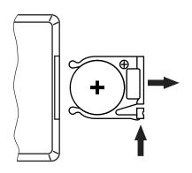
Push the lock of the battery holder towards the centre of the housing and pull out the battery holder like a drawer. Insert the batteries. The battery is correct if the positive pole points to the housing base of the remote control. Slide the battery holder back into the remote until it clicks into place.
